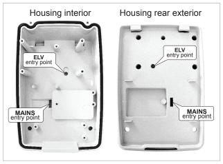
ensure LV and ELV cables are segregated. Locate the enclosure base over the all mount base with the top 2 lugs and bottom screws provided.
